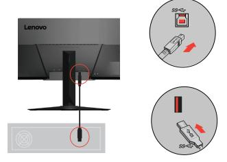
8. Connect one end of the USB cable to the USB downstream terminal on the side of the monitor, and connect the other end of the USB cable to an appropriate USB port on your device.
