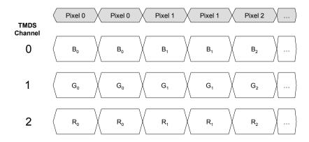
Figure 6-4 RGB with Pixel-Doubling
