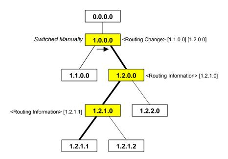
CEC Figure 11 Example message flow, when a CEC Switch is manually switched
