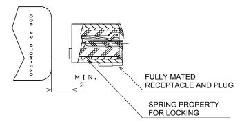
Figure 4-6 Type B Receptacle and Plug Mated Condition
