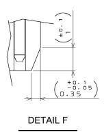
• The form shown above is required. This feature will reduce the likelihood of damage to the receptacle insulator under rough operation.
