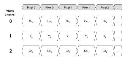
Figure 6-6 YC<sub>B</sub>C<sub>R</sub> 4:4:4 with Pixel-Doubling
