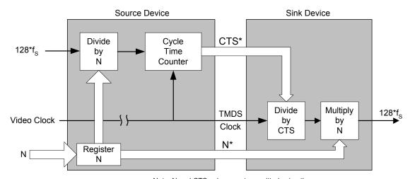
Note: N and CTS values are transmitted using the "Audio Clock Regeneration" Packet. Video Clock is transmitted on TMDS Clock Chanel.
