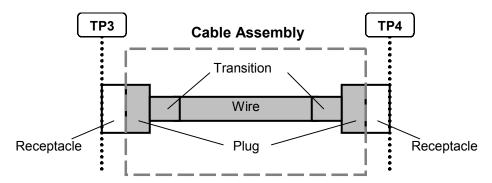
Figure 4-15 Cable Assembly Test Points
