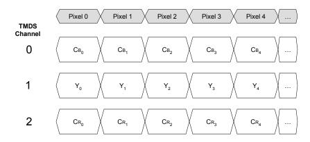
Figure 6-3 8-bit YCBCR 4:4:4 mapping
