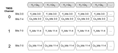
Figure 6-2 YC<sub>B</sub>C<sub>R</sub> 4:2:2 component
