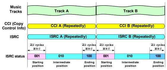
Figure 8-4 ISRC/CCI and ISRC Status Handling
