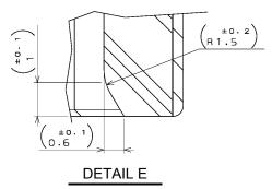
The form shown above is required. This feature will reduce the likelihood of damage to the receptacle insulator under rough operation.
