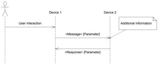
CEC Figure 2 Example Message Flow Diagram
