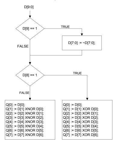
Figure 5-7 TMDS Video Decode Algorithm
