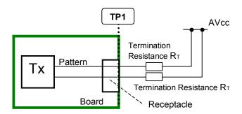
Figure 4-11 Balanced Source Test Load
