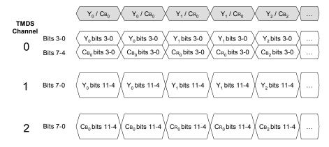
Figure 6-5 YC<sub>B</sub>C<sub>R</sub> 4:2:2 with Pixel-Doubling
