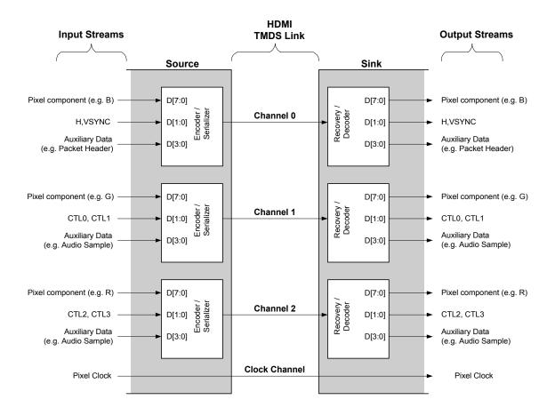
Figure 5-1 HDMI Encoder/Decoder Overview
