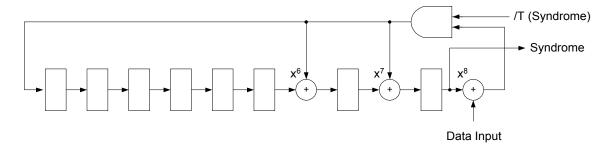
Figure 5-5 Error Correction Code generator
