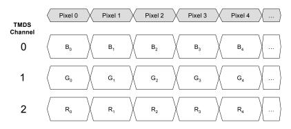
Figure 6-1 Default pixel encoding: RGB 4:4:4, 8 bits/component
