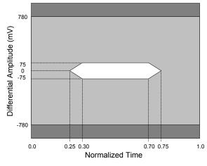
Figure 4-14 Absolute Eye Diagram Mask at TP2 for Sink Requirements
