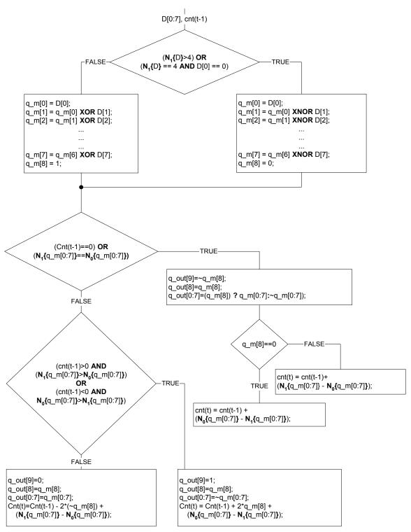
Figure 5-6 TMDS Video Data Encode Algorithm
