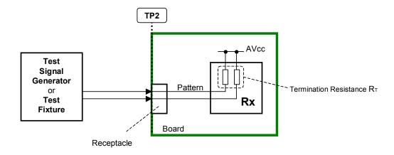
Figure 4-13 HDMI Sink Test Points
