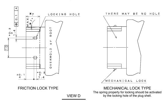
Figure 4-5 Type B Plug Mating Interface Dimensions
