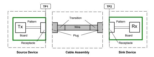
Figure 4-10 TMDS Link Test Points
