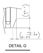
The form shown above is required. This feature will reduce the likelihood of damage to the receptacle insulator under rough operation.
