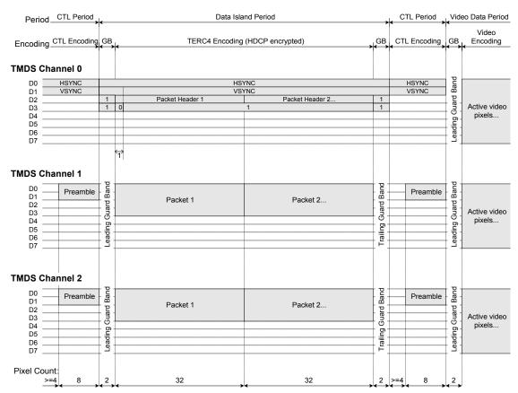
Figure 5-3 TMDS Periods and Encoding
