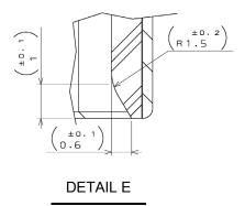
The form shown above is required. This feature will reduce the likelihood of damage to the receptacle insulator under rough operation.
