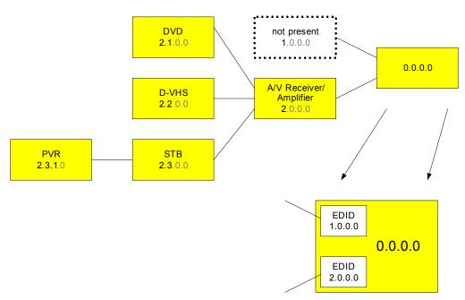
Figure 8-3 Addresses within an HDMI cluster
