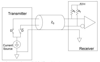
Figure 4-7 Conceptual Schematic for one TMDS differential pair
