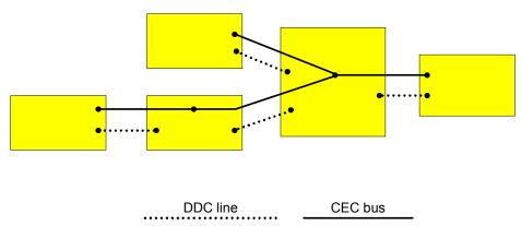
Figure 8-1 CEC and DDC line connections
