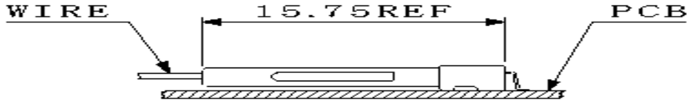
Figure 4-52: Mating Condition (Reference) of Panel Side Internal Cable Connector (mm)
